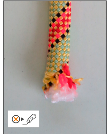
• Damaged rope end
