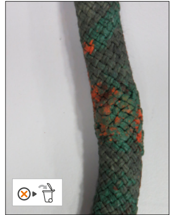
• Trace of paint
