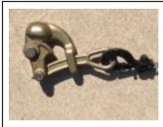
**Havens® grip**—This product manufactured by Klein Tools is a camming device used to secure a cable or rope to a second cable. The Havens grip is often used along with a chain puller or ratchet winch to tighten a cable.
