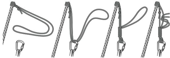
The mariner's knot is a hitch made by wrapping cordage between two carabiners. The mariner's knot can be released while under load. This is useful when transferring a load between two different anchors, such as passing a knot or during a belay escape.
