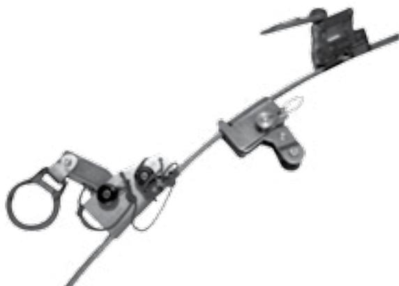
manually pushed up the cable as the instructor climbs. This must be done by lifting the tether or carabiner. Never hold the body of the ascender. Keeping the ascender at chest level will limit the dropping distance in the event of a fall.
