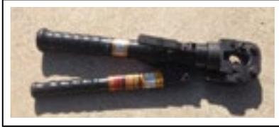
**Cable cutter**—A quality cable cutter will cleanly sever a cable so that it can be used with cable fittings. For COPE course construction, select one made to cut 3/8-inch 7x19 aircraft cable. The cutter can be manual or hydraulic.
